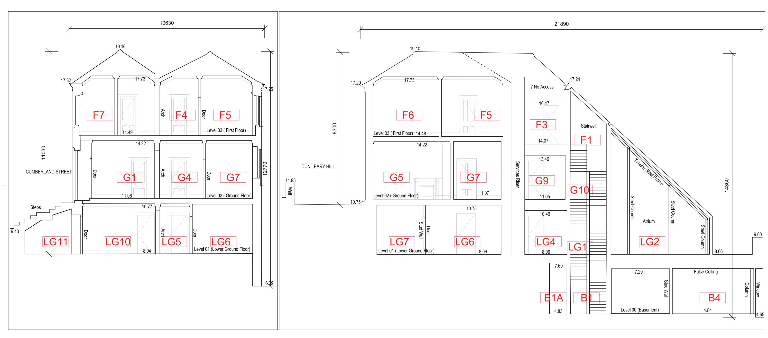
Cross-Section A-A Cross-Section B-B
