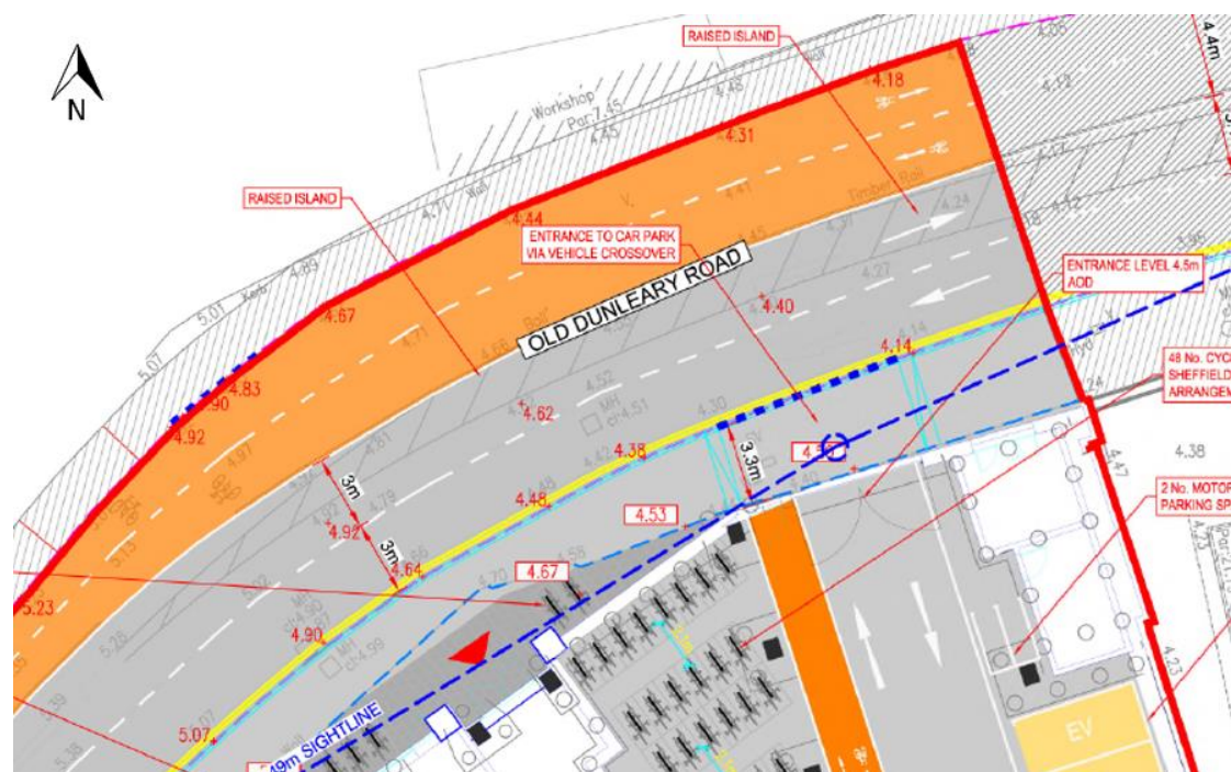
Figure 3.6: Vehicular Site Access Sight Line Drawing
